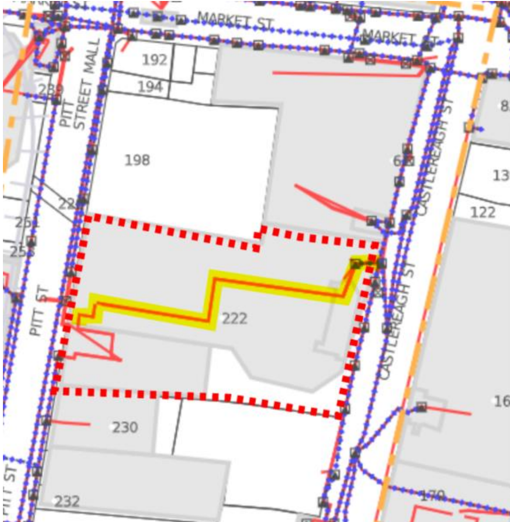
Figure 5: Optus existing Communications Services adjacent the site
